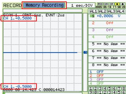
When the blocks in the memory block capture display section and the event data display section are filled with color, this indicates that event data has been captured.
